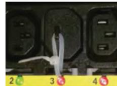
Cap secures in place with cable tie
